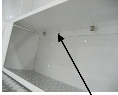
Use under seat flange holes to mark and Drill through front bulkhead with 1/4" bit. Use 1/4" x 3/4" bolts and serrated to attach seat to bulkhead.
